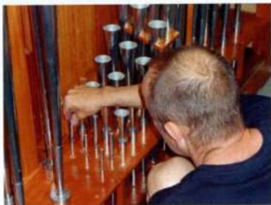
Tomasz Nowak installing and tuning the new trumpet rank. Each pipe is cut to exact length.
