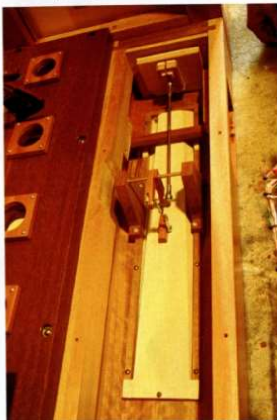
The reed chest regulator keeps the pressure at 60mm WG by means of a large pneumatic motor which actions a regulating valve
